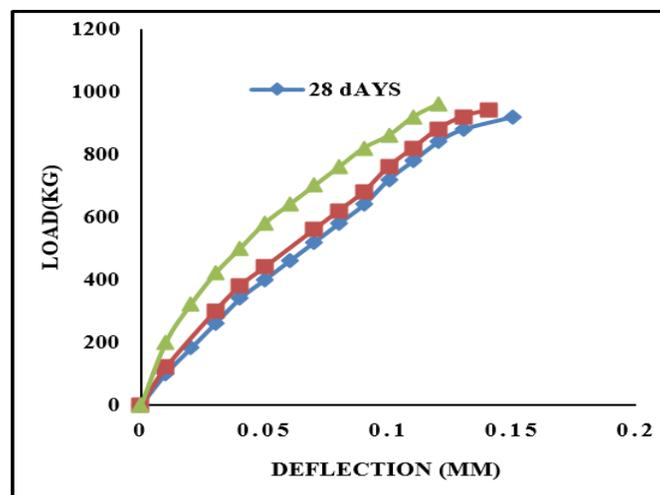
Figure 6: Load vs. Deflection curve for WFS20%
