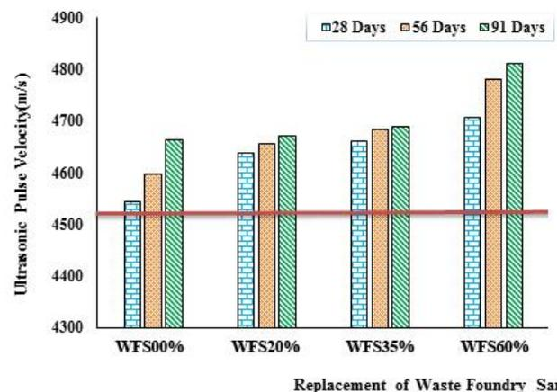
Figure 4: Variation of ultrasonic Pulse velocity with Replacement (%) of WFS
