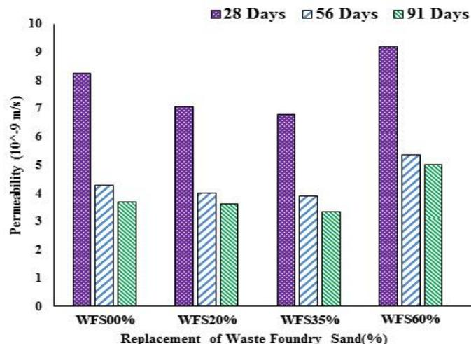
Figure 9: Variation of Coefficient of Permeability with % replacement of WFS
