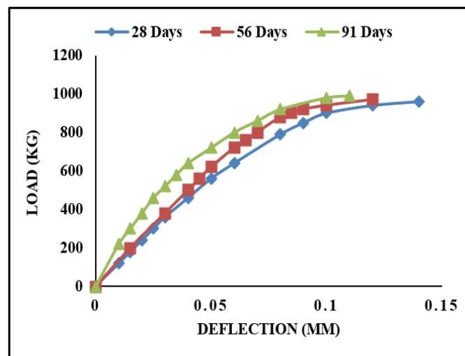
Figure 7: Load vs. Deflection curve for WFS35%
